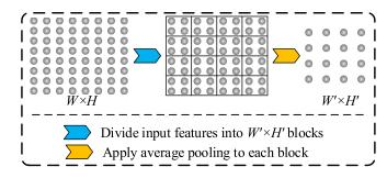
Fig. 9. Illustration of the adaptive average pooling in the proposed FSM.
