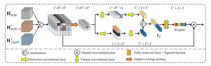
Fig. 7. Architecture of our proposed FSM. First, an adaptive average pooling is employed on concatenated cross-modal and unimodal features to squeeze the spatial information of input features into channel descriptors. Then, these channel descriptors are fed into two parallel branches with mirrored structures for aggregating local information to global information. Finally, weights for different channels of cross-modal and unimodal features are generated by a fully connected layer.
