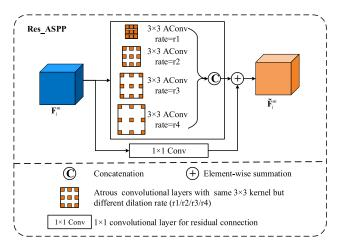
Fig. 4. Architecture of Res\_ASPP. In Res\_ASPP, four parallel atrous convolutional layers with different dilation rates are first employed to extract multi-scale features. Then, a short connection path is employed as a residual mapping. Finally, the outputs of Res\_ASPP are obtained by adding the extracted multi-scale features and the features from the short connection path.
