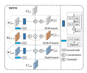
Fig. 5. Diagram of the proposed MFFM. The proposed MFFM contains three branches, one branch for capturing cross-modal complementary information while the other two branches for preserving unimodal (RGB and depth) features to the next stage.
